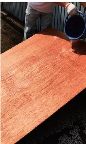
Adding a water-repellent and moisture-proof function on the front and back reduces plywood deterioration!
